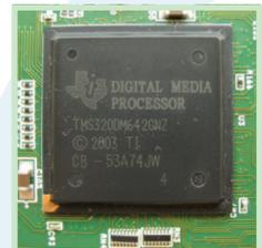
Paying close attention to software architecture design and performance optimization resulted in record-breaking utilization of hardware resources. When decoding three 512x384 video streams received over network, with resize and rotate functions on three full XGA video outputs, the software consumes about 95 percent of CPU running at 600 MHz.
